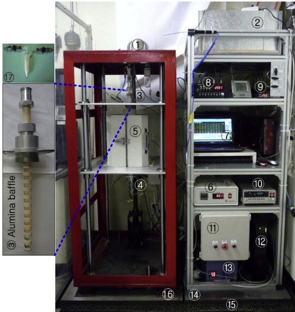
Fig. 2. Experimental set-up of thermogravimetric analysis (TGA) with Cahn microbalance D-200.
